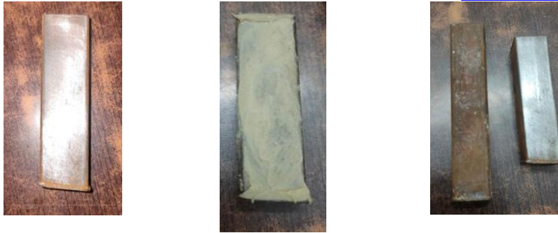
Normal Iron After coating of grease Effect of grease Figure 5: Effect of grease coating on metal surface
