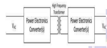
When SSTs are implemented, they will radically change the way utility power is distributed. They will also become integral components in the future Smart Grid - enabling it to direct power from any source to any destination by the most efficient route possible.
