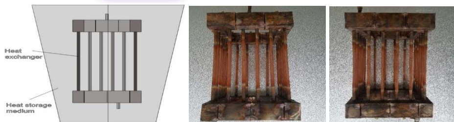
Figure 3. Heat exchanger: a) heat exchanger-heat storage ensemble; b) images of the real model.
