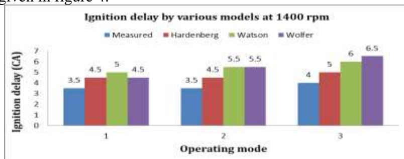
Figure 4: Ignitin Delay period using different models at 1400 rpm
