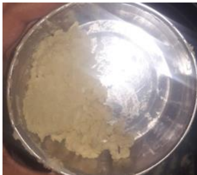
Figure 3: Calcium stearate-based greases
