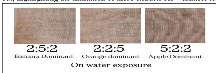
Figure 2: Fading and Blotchiness after water immersion
