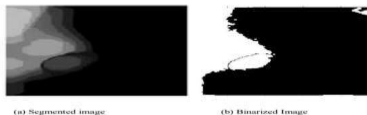
Figure: Result after Binarization process using thresholding method.
